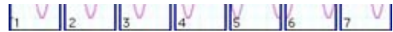
Graph 3.4: Our signal of 3.2 now split into 7 frames. Each frame will be passed to our transform and be analyzed. We see that while the signal in 3.3 nicely fits into the frames, the second signal appears to have a phase shift in each window (click to enlarge).
